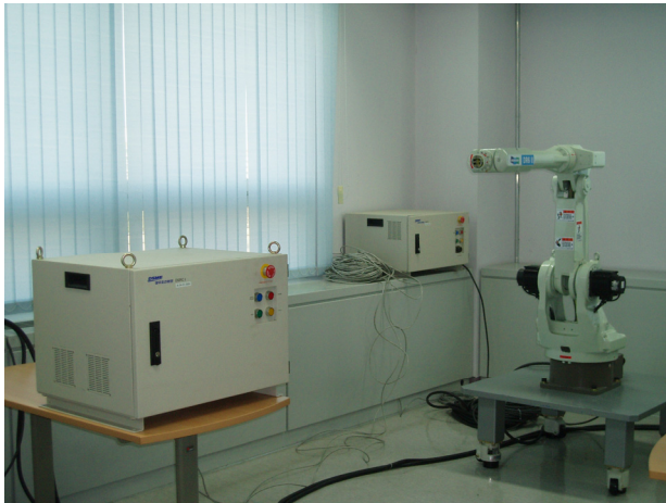
Fig. 1 DSME controller and robot: The box in left side is main control part and the box near robot is servo control part.
